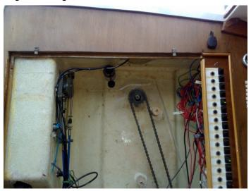
To the right, you can see the switch panel that I fitted some years ago. This is simply made of plywood, I glued and pinned some "L" shaped battens around the edge of the original hole so that the panel then slides in and out for maintance (from the left).
