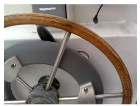
The Autohelm drive unit is fitted conventionally to the wheel, with three fittings on my six spoke wheel. In the background, you can see the Control unit, which has been fitted in a GlassFibre box.
