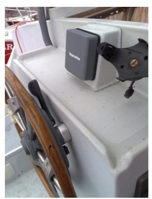
Aaron at Hayling Marine Services made me the glassfibre box for the autohelm control, and also glassed in the hole where the compass was. With his usual skill it is now impossible to see where the compass was.
